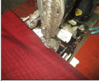
Photo of non-conformity Needle Guard Not Provided.JPG
